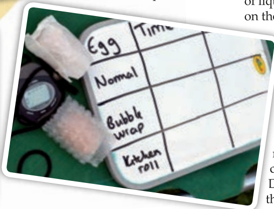
Figure 6 Measuring and recording how long hard-boiled eggs covered in different materials take to roll down a ramp
